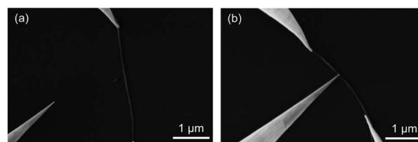
Fig. 1 SEM images of (a) 2 tungsten probes on an isolated MWCNT and (b) 3 tungsten probes on an isolated MWCNT with the centre probe floating.
