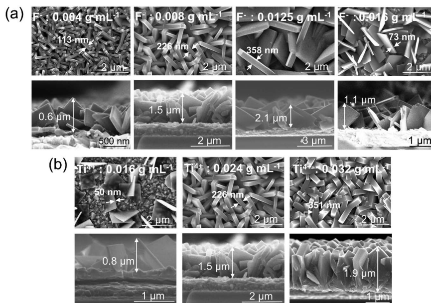
Fig. 1 Top view and cross-sectional SEM images of TiO 2 nanosheets grown on FTO using (a) different concentrations of F precursor, (b) different concentrations of Ti precursor.
