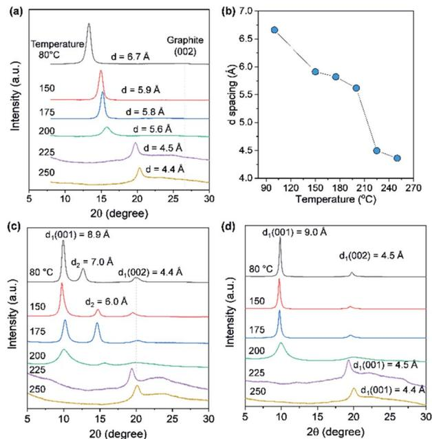
Fig. 5 (a) X-ray diffraction patterns and (b)  $d$ -spacing of AGO films upon thermal treatment at different temperatures for 1 h. (c and d) XRD patterns of thermally treated AGO films after immersing in EtOH for (c) 3 h and (d) 15 h.
