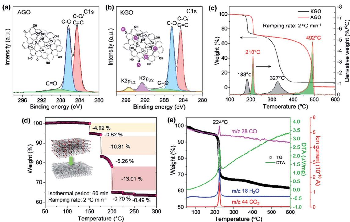
Fig. 3 C 1s XPS spectra of (a) AGO and (b) KGO. (c) TGA results for AGO and KGO in air. (d) Isothermal thermogram in air for AGO at 150, 175, 200, 225, and 250  $^\circ\text{C}$  for 60 min; the ramping rate at each step is  $2^\circ\text{C min}^{-1}$ . (e) TGA-MS data of AGO under an Ar environment showing  $\text{H}_2\text{O}$  ( $m/z$  18),  $\text{CO}$  ( $m/z$  28), and  $\text{CO}_2$  ( $m/z$  44).
