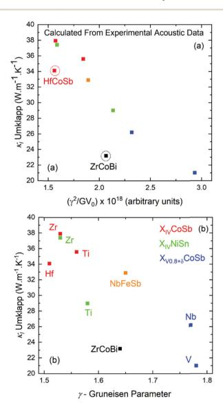
Fig. 3 Plots of calculated lattice thermal conductivity ( $\kappa_{\rm l}$ ) at 300 K (see Section 2.4), assuming the presence of only Umklapp scattering (i.e. for the defect free parent materials), versus (a) the variables determining the magnitude of Umklapp scattering and (b) the acoustic Grüneisen parameter. HfCoSb and ZrCoBi have lower  $\kappa_{\rm l}$  due to low  $v_{\rm s}$  (see Table 2).
