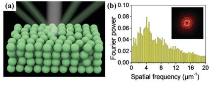
Fig. 1 (a) Schematic of an amorphous colloidal array under white light, and the structural colour from the amorphous array remains nearly unchanged depending on the viewing angle. (b) Histogram of two-dimensional RDF of the APC structure; inset is the 2D Fourier transform. (Reproduced with permission.<sup>36</sup> Copyright 2018, American Chemical Society.)
