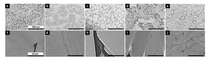
Fig. 2 SEM images of MAPb<sub>0.5</sub>Sn<sub>0.5</sub>I<sub>3</sub> with 0% (a; f), 0.1% (b; g), 0.2% (c; h), 1% (d; i) and 5% (e; j) F4TCNQ dopant, using an Everhart–Thornley detector with  $100 \times$  magnification (a to e) and a Trinity detector with  $5000 \times$  magnification collecting mostly secondary electrons (f to j). The scale bar is  $500 \mu$ m for (a) to (e) and 10  $\mu$ m for (f) to (j).
