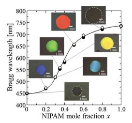
Fig. 3 Plots of the Bragg wavelength and photographs of the elastomer-immobilized colloidal crystal films as a function of x ( $\bullet$ : experimentally measured Bragg wavelength,  $\diamond$ : calculated Bragg wavelength).
