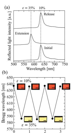
Fig. 5 (a) Spectral change of the elastomer-immobilized colloidal crystal film with x = 0.50 by repeating the stretch and release. (b) Photographs and Bragg wavelength of the film by repeating the stretch and release 3 times. The length of the scale bars is 5.0 mm.
