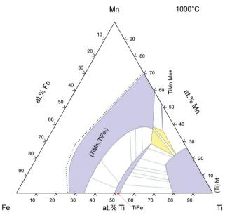
Isotherm section at 1000 °C of the Ti-Fe-Mn phase diagram. Reproduced with permission from ref. 22.
