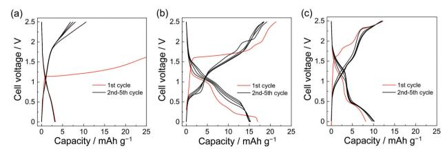
Fig. 4 Charge-discharge performance of symmetric NiNc-NiNc batteries assembled with distinct electrolytes: (a) EC/DMC, (b)  $[C_2C_1im][FSA]$ , and (c) 50 mol% Na[FSA]-[C<sub>2</sub>C<sub>1</sub>im][FSA]. Current density and cut-off voltages were set as 50 mA  $g^{-1}$  and 0–2.5 V.
