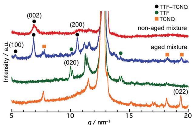
Fig. 3 XRD patterns of the non-aged mixture (red line), aged mixture (blue line), aged TTF crystal (green line), and aged TCNQ crystal (orange line). The diffraction peaks at  $11.5 \text{ nm}^{-1}$  and  $12.8 \text{ nm}^{-1}$  indicate the diffraction from the filter.
