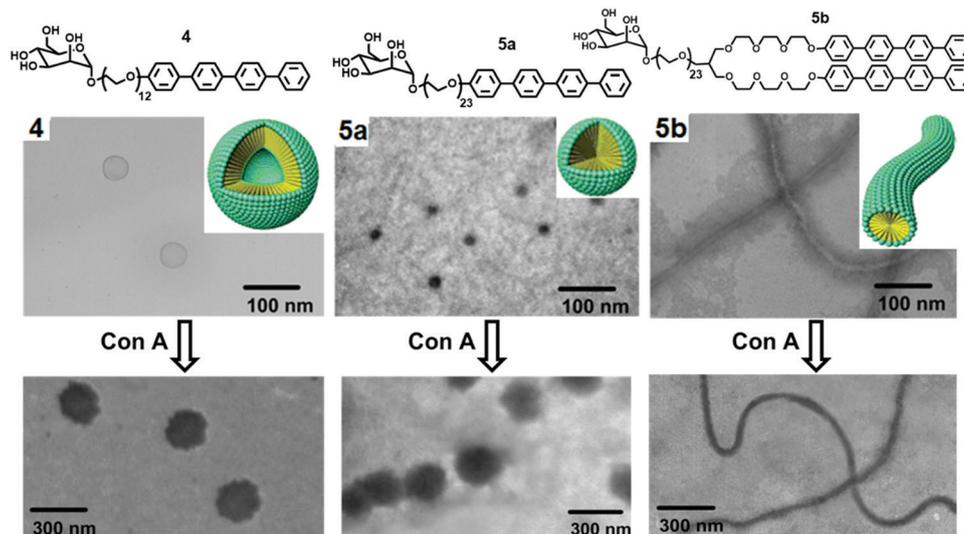
Fig. 5 Molecular structures of mannose and galactose functionalized amphiphiles **4**, **5a** and **5b** and schematic representation of their self-assembly into distinct nanostructures and their corresponding TEM images before and after interaction with Con A. Adapted with permission from ref. 33. Copyright 2005 American Chemical Society.
