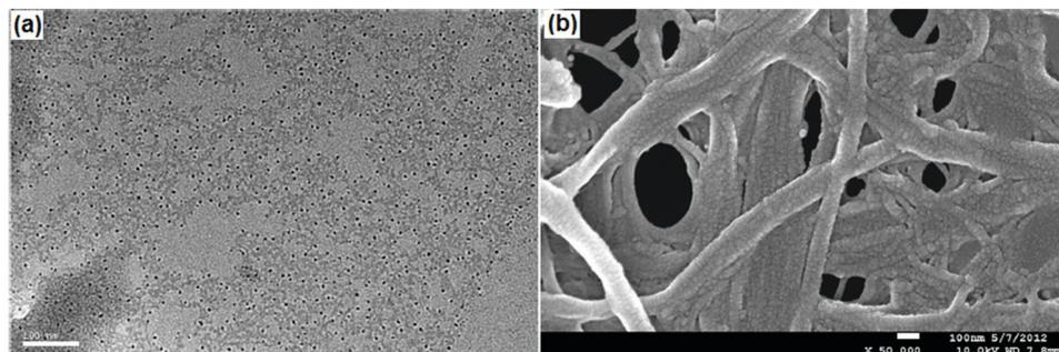
Fig. 10 Schematic representation of possible self-assembly mode of compound **10** and interaction with Con A. (a) TEM and (b) SEM images of the complexes formed between the self-assembled structure of compound **10** and Con A. Reprinted with permission from ref. 38. Copyright 2013 Royal Society of Chemistry.
