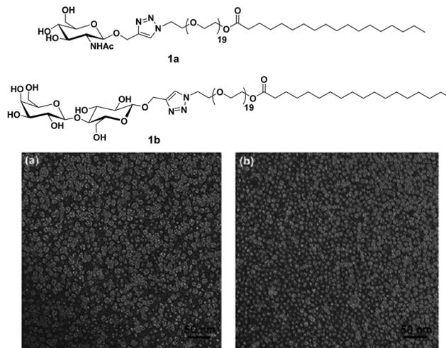
Fig. 1 Molecular structures of amphiphiles and TEM images of amphiphiles **1a** and **1b** showing spherical micelles of size around 10 nm. Reprinted with permission from ref. 29. Copyright 2011 Royal Society of Chemistry.
