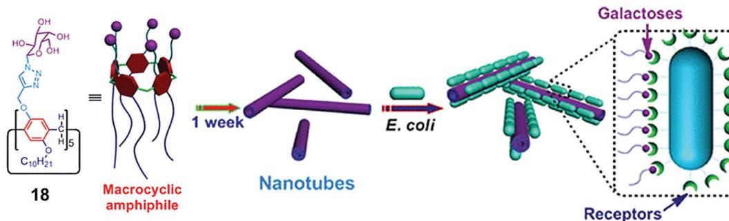
Fig. 18 Molecular structure of pillar[5]arene amphiphile (**18**) and schematic representation of its transformation into nanotubes and interaction with *E. coli*. Reprinted with permission from ref. 47. Copyright 2013 American Chemical Society.
