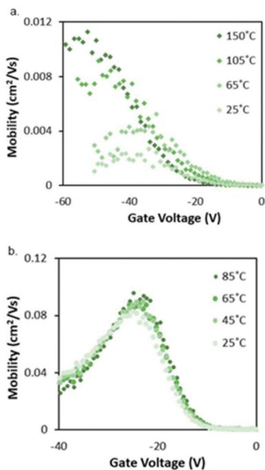
Fig. 9 Characterisation of Cl-AlPc OTFTs. (a)  $V_{GS}$  vs.  $\mu$  curves at temperatures ranging from 25 °C to 150 °C in vacuum. (b)  $V_{GS}$  vs.  $\mu$  curves at temperatures ranging from 25 °C to 85 °C in air. Reproduced from ref. 33 with permission from The Royal Society of Chemistry.
