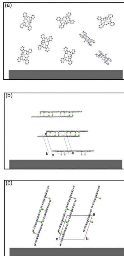
Fig. 13 Schematic molecular packing of a Cl-AlPc (CCDC: 1134071) film fabricated on a pure SiO<sub>2</sub> substrate at room temperature (a) and 120 °C (b), and on an OTS-modified surface at 120 °C (c). The image is reprinted with permission from ref. 163. Copyright 2011, Wiley-VCH.
