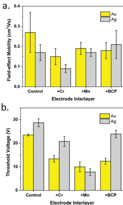
**Fig. 17** Saturation region properties for OTFTs using  $(F_5PhO)_2$ -SiPc as the semiconductor layer with Au and Ag electrodes and Cr, Mn, or BCP interlayers: (a) field-effect mobility and (b) threshold voltage. Reprinted with permission from ref. 34. Copyright 2020, American Chemical Society.
