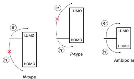
Fig. 7 The compatible relationship between the work function of S/D electrodes and the HOMO/LUMO of the semiconductor material.
