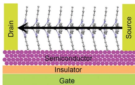
**Fig. 18** The favourable molecular orientation of PbPc in OFETs. The arrows indicate the direction of the highest electrical conductivity. Reprinted figure with permission from ref. 164 Copyright @ 2012, World Scientific.
