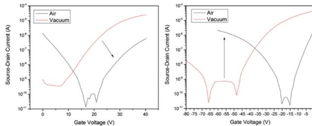
Fig. 15 Sample transfer curves for OTFTs using  $(\text{F}_5\text{PhO})_2\text{-SiPc}$  as the active layer when operated in the electron accumulation region (left) and hole accumulation region (right) and characterised either under vacuum or in air. The image is reprinted with permission from 38. Copyright 2019, Wiley-VCH.
