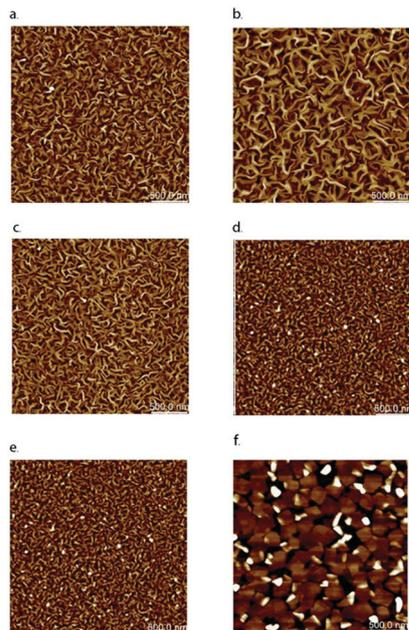
Fig. 11 AFM images (2.5 mm × 2.5 mm) of (a) CuPc (b) FePc (c) CoPc (d) ZnPc (e) MgPc (f) Cl-AlPc deposited on heated silicon substrates. Reproduced from ref. 33 with permission from The Royal Society of Chemistry.
