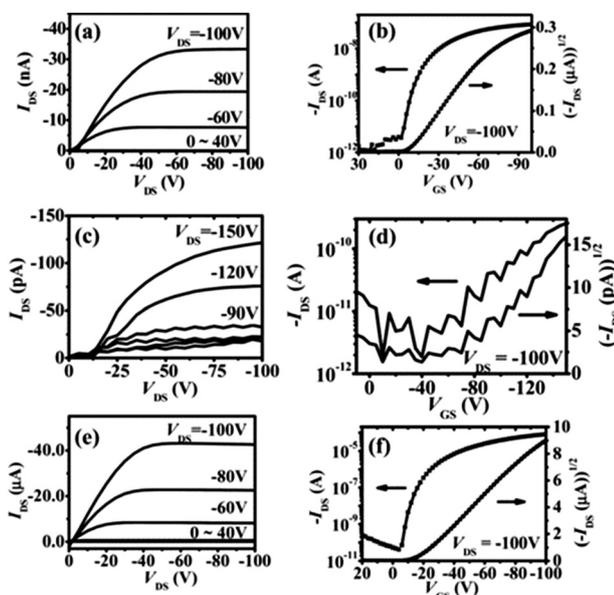
Fig. 12 Output and transfer curves of devices with Cl-AlPc active layer fabricated under different conditions: (a and b) pure SiO<sub>2</sub> surface at room temperature; (c and d) pure SiO<sub>2</sub> surface at 120 °C; (e and f) OTS-modified surface at 120 °C. The image is reprinted with permission from ref. 163. Copyright 2011, Wiley-VCH.
