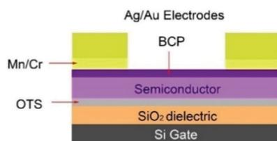
**Fig. 16** Device schematic for TC/BG OTFTs with either an electron transport (bathocuproine (BCP)) or low-work-function metal (Mn/Cr) interlayer between the main electrode (Ag/Au) and organic semiconductor. Reprinted with permission from ref. 34. Copyright 2020, American Chemical Society.
