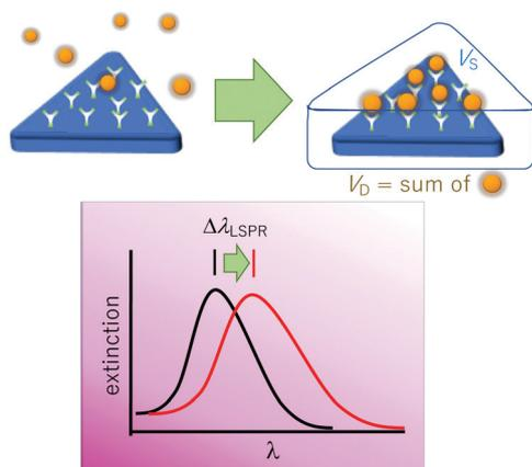
**Fig. 6** Nanoprism sensor based on refractive index changes. Binding of analyte species (spheres) within the sensing volume ( $V_s$ ) causes the change of effective refractive index in the immediate vicinity, resulting in an LSPR shift ( $\lambda_{\text{LSPR}}$ ).
