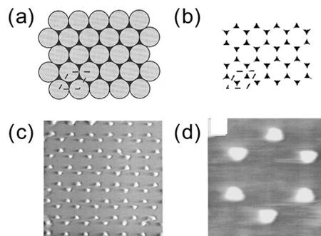
Fig. 5 NSL. (a) Spin-coated polystyrene nanospheres (grey) and vapor deposited metal (black). (b) After the removal of the nanospheres. (c) AFM image ( $1.7 \times 1.7 \mu m^2$ ). (d) AFM image ( $470 \times 470 nm^2$ ). Reprinted with permission from J. C. Hulteen and R. P. Van Duyne, *J. Vac. Sci. Technol., A*, 1995, **13**, 1553–1558. Copyright (1995), American Vacuum Society.<sup>59</sup>
