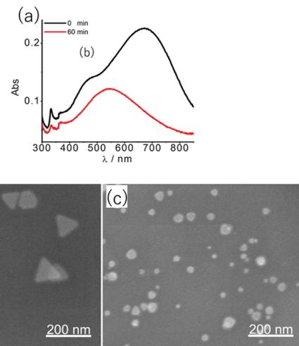
Fig. 8 Changes in absorption spectra (a) as Ag NPRs were etched from (b) to (c) by  $\text{H}_2\text{O}_2$  produced by GOx-catalysed oxidation of glucose. Reprinted with permission from Y. Xia *et al.*, *Anal. Chem.*, 2013, **85**, 6241–6247. Copyright (2013) American Chemical Society.<sup>75</sup>
