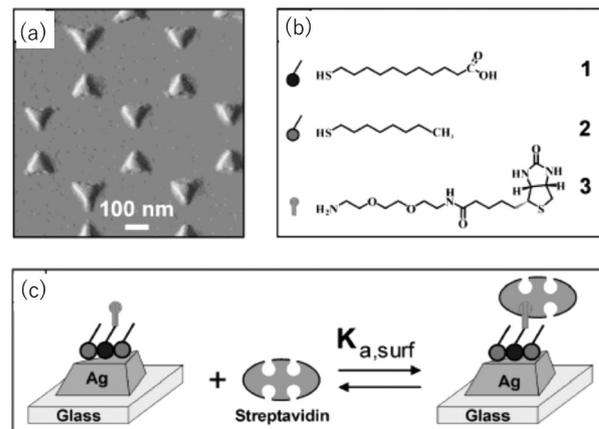
Fig. 7 Ag nanoprism array sensor for streptavidin. (a) AFM image. (b) Compounds used. (c) Binding of streptavidin to the sensor. Reprinted with permission from A. J. Haes and R. P. Van Duyne, *J. Am. Chem. Soc.*, 2002, **124**, 10596–10604. Copyright (2002) American Chemical Society.
