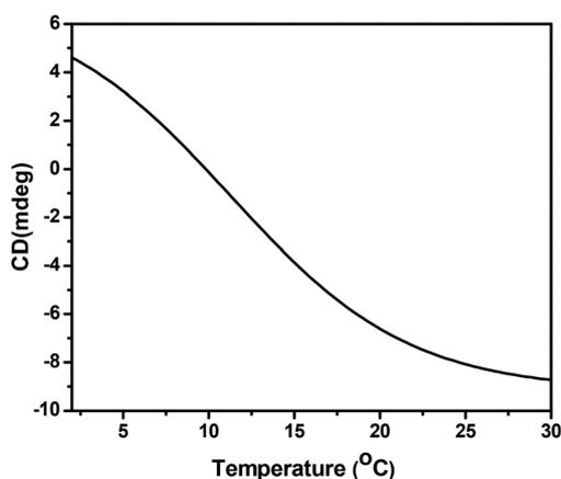
Fig. 6 Thermal denaturation curve of collagen type I from codfish skins extracted using an aqueous solution of U:LA (1:2) at 222 nm; heating rate of 0.1 °C min<sup>-1</sup>.
