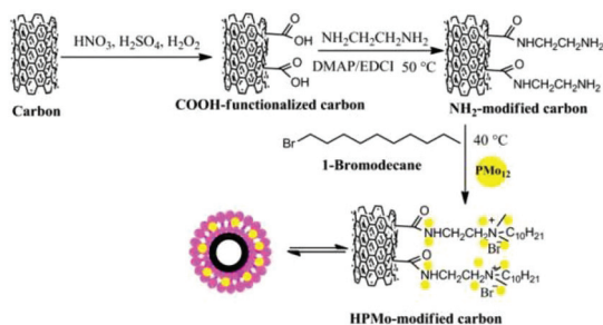
Fig. 12 Synthetic progress of HPMo-modified carbon catalysts. 149 Reproduced from ref. 149 with permission from WILEY, copyright 2015.
