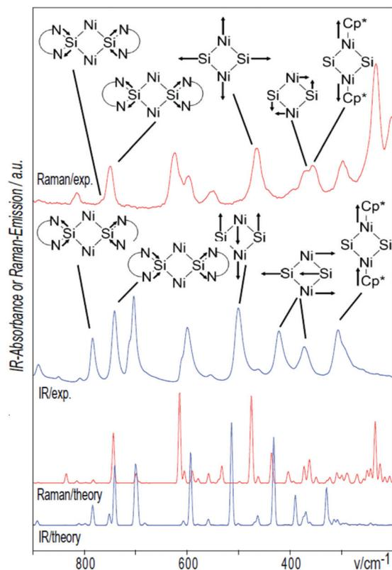
Fig. 2 Experimental and theoretical IR and Raman spectra of the title compound. The normal modes of the molecular framework are given.
