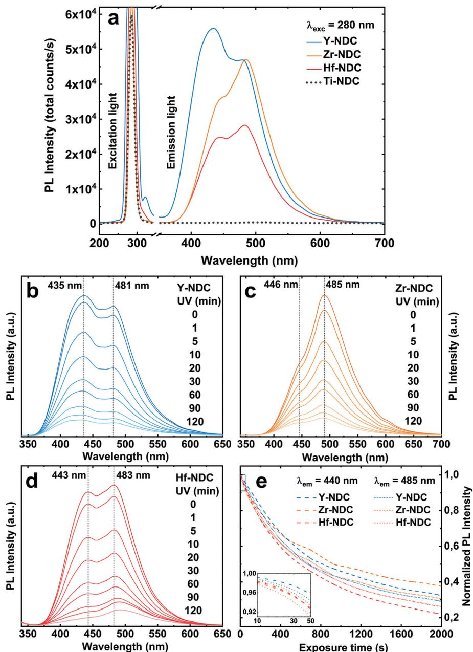
Fig. 7 (a) Photoluminescence emission spectra of the hybrid films: Ti-NDC (100 nm), Zr-NDC (109 nm), Hf-NDC (108 nm) and Y-NDC (99 nm). PL was recorded using a 280 nm diode. (b–d) The time evolution of the PL spectra upon UV exposure. (e) Normalized PL intensity of the two emission peaks at 440 nm and 485 nm vs. UV exposure time. The inset shows a zoomed-in view of the first 50 s on a logarithmic scale.
