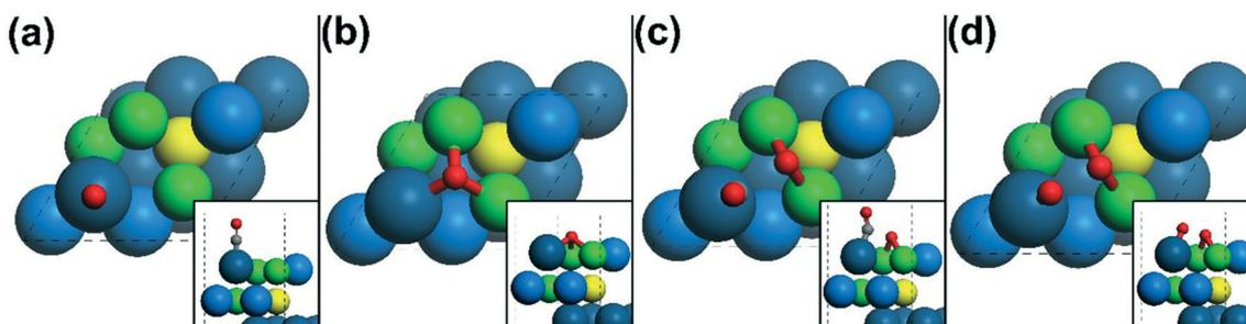
Fig. 6 The top views and side views (insets) of (a) adsorbed CO, (b) adsorbed oxygen atoms, (c) transition state of CO oxidation, and (d) transition state of  $\text{O}_2$  dissociation on the catalyst candidate of step 9. Oxygen and carbon atoms are in red and grey, respectively.
