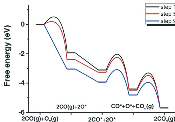
**Fig. 5** The energy profiles of CO oxidation on the catalysts of step 1 (black), step 5 (red) and step 9 (blue) in the free energy landscape.
