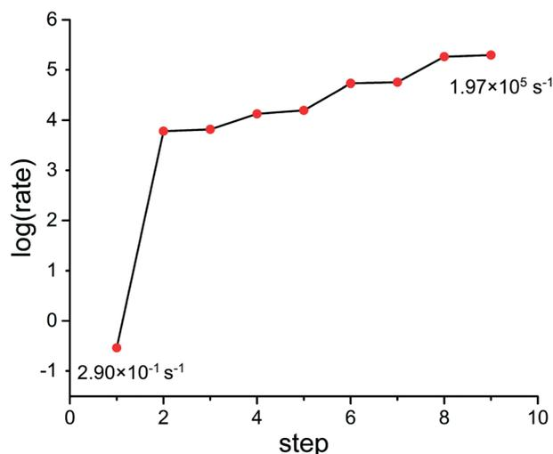
Fig. 3 The activity change of CO oxidation on the catalysts designed in steps 1 to 9. The activities increase from  $2.90 \times 10^{-1} \text{ s}^{-1}$  of step 1 to  $1.97 \times 10^5 \text{ s}^{-1}$  in our design process.
