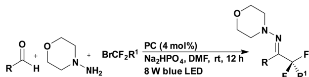
Fig. 43 Reaction scheme for the coupling of aldehydes with hydrazines and bromodifluorinated reagents.
