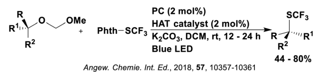
Fig. 199 Reaction scheme for the trifluoromethylthiolation of tertiary ethers.
