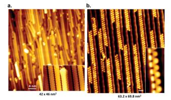
**Fig. 12** STM images of aligned graphene nanoribbons on Au(788), scale bars 4 nm. (a) 7-AGNR and (b) cGNRs (**31**). Reprinted figure with permission from ref. 77. Copyright 2012 by the American Physical Society.
