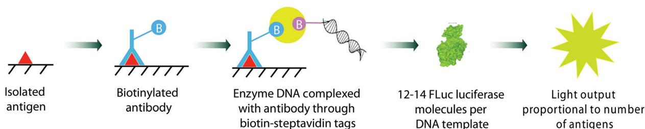
Fig. 11 The gene expression immunoassay for detection of prostate specific antigen (PSA) reported by Christopoulos *et al.*<sup>264</sup>
