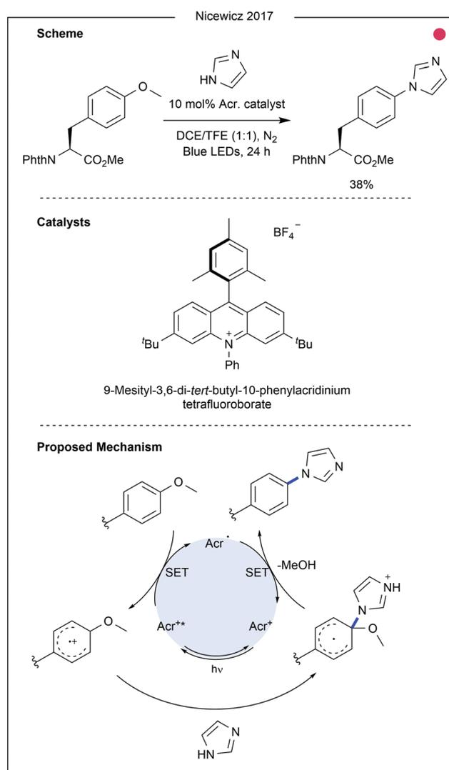
**Fig. 18** Tyrosine methyl ether activated for  $\text{S}_{\text{N}}\text{Ar}$  reactivity through the use of an acridinium photocatalyst. After oxidation of the tyrosine aryl ring by the photocatalyst, imidazole was shown to attack. Reduction occurred with loss of methanol to generate the product. Phth = phthaloyl. Acr. = 9-mesityl-3,6-di-*tert*-butyl-10-phenylacridinium tetrafluoroborate. DCE = dichloroethane. TFE = trifluoroethanol.
