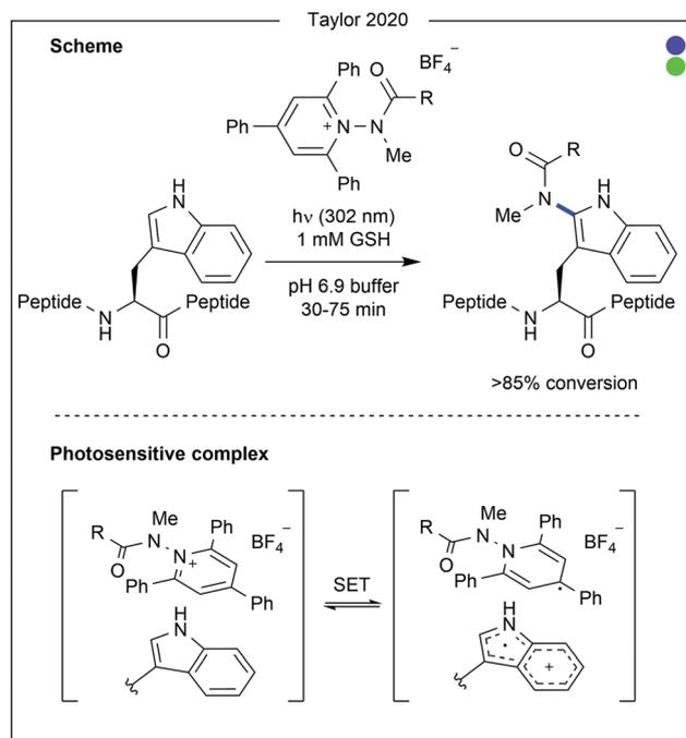
Fig. 16 Photo-induced modification of tryptophan at the C<sub>2</sub>-position. The photosensitive complex undergoes single electron transfer when irradiated by ultraviolet light, leading to scission of the N-N bond in the Katritzky-type salt. Radical combination then generates the final product. GSH = glutathione.
