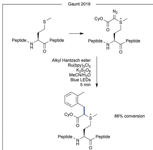
**Fig. 11** Photocatalysis for further modification of a protein after initial handle attachment to methionine. A C<sub>4</sub>-substituted Hantzsch ester releases a benzyl radical after photocatalytic oxidation. After cleavage of the pendant diazo group on the peptide, the two radicals can combine to form the further modified product. Bpy = 2,2'-bipyridyl.
