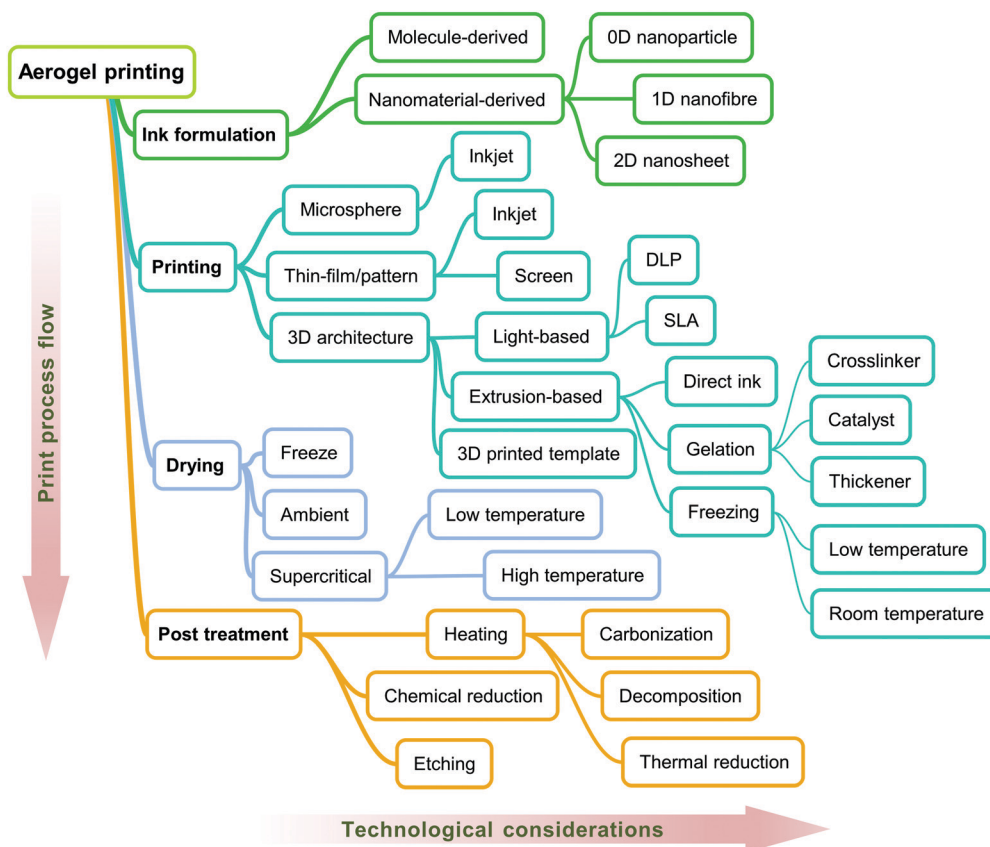
Fig. 5 Relevant technical considerations for aerogel printing.
