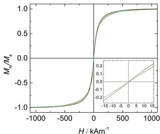
Fig. 4 Magnetization curves of a dried  $\text{CA@Fe}_3\text{O}_4$  particles (—),  $\text{CA@Fe}_3\text{O}_4$  particles dispersed in water (—) and 9OCB-PHMS@ $\text{Fe}_3\text{O}_4$  particles in 5CB (—).
