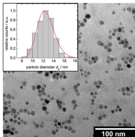
Fig. 3 TEM image and corresponding size histogram of CA@Fe<sub>3</sub>O<sub>4</sub> nanoparticles with a log normal distribution function (—).
