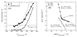
Fig. 7 Temperature dependencies of catalytic activity with or without electric field (EF). (A) Activities for catalytic steam reforming by heat (SR) and applying EF (ER); (B) Arrhenius plots for both reactions, preset temperature, 398-823 K; catalyst, 1.0 wt% Pd/CeO<sub>2</sub>, 80 mg; flow, CH<sub>4</sub>:  $H_2O: Ar: He = 12: 24: 12: 72$ , total flow rate 120 sccm; current, 0 or 5 mA. Reproduced with permission from literature.<sup>34</sup>
