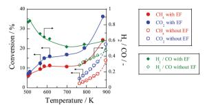
Fig. 10 Temperature dependence for catalytic activities with EF over 0.88 wt% Ni/10 mol% La-ZrO<sub>2</sub> catalyst, CH<sub>4</sub>: CO<sub>2</sub>: Ar = 1:1:2, total flow rate: 20-200 sccm; input current: 3 mA; catalyst weight: 100 mg; furnace temperature: 505-880 K (with EF) and 764-897 K (without EF). Reproduced with permission from literature.40
