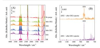
Fig. 13 Operando-DRIFTS spectra with/without EF. (A) Comparison of before/with/after applying EF (without EF, DR; with EF, ER). (B) Differential spectra with/after applying EF in H $_2$ O rotation: 0.88 wt% Ni/10 mol% La–ZrO $_2$  catalyst; CH $_4$ : CO $_2$ : He = 3:3:34; 40 Sccm total flow rate; 9 mA current; 573 K preset temperature. Reproduced with permission from literature. $^{40}$
