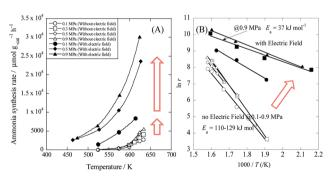
Fig. 4 Temperature and pressure dependence of ammonia synthesis rate with/without an electric field. (A) Temperature dependence of the ammonia synthesis rate at 0.1–0.9 MPa. (B) Arrhenius plots for each reaction: catalyst bed temperature, 463–634 K; catalyst, Cs/Ru/SrZrO $_3$ , 200 mg; flow, N $_2$ : H $_2$  = 1:3, total 240 sccm; current, 0 or 6 mA. Reproduced with permission from literature. <sup>42</sup>
