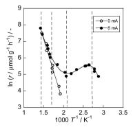
Fig. 6 Arrhenius plots for NH<sub>3</sub> synthesis rate (r) over 1 wt% Ru/CeO<sub>2</sub> with/ without an electric field (0 or 6 mA) under  $P_{\rm H_2}$  = 0.75 atm. Reproduced with permission from literature.72
