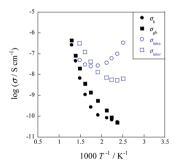
Fig. 9 Electrical conductivity of porous CeO<sub>2</sub> as a function of inverse temperature under dry and wet conditions ( $P_{H_2O}$  = 0.026 atm). Reproduced with permission from literature.<sup>78</sup>
