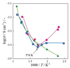
Fig. 11 Logarithmic apparent electrical conductivity as a function of inverse temperature with EF over 0.88 wt% Ni/10 mol% La-ZrO<sub>2</sub> catalyst,  $CH_4$  (or  $CD_4$ ):  $CO_2$ : Ar = 1:1:2 or  $CO_2$ : Ar = 1:3; total flow rate, 100 sccm; 3.0 mA input current; 100 mg catalyst weight; 404-856 K catalyst bed temperature. Reproduced with permission from literature. 40
