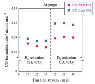
Fig. 12 CO formation rate with the EF over 0.88 wt% Ni/10 mol% La–ZrO $_2$  catalyst, CH $_4$  (or CD $_4$ ): CO $_2$ : Ar = 1:1:2; total flow rate, 100 sccm; 3.0 mA input current; 100 mg catalyst weight; 423 K furnace temperature. Reproduced with permission from literature.  $^{40}$
