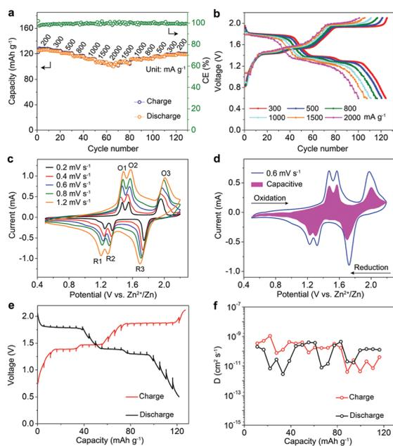
**Fig. 3** (a) Rate performance and (b) corresponding voltage profiles of the LVP cathode in 1 m Zn + 15 m Li electrolyte. (c) CV curves and (d) typical capacitive contribution at 0.6  $\text{mV s}^{-1}$ . (e) GITT profiles and (f) corresponding ion diffusion coefficient.
