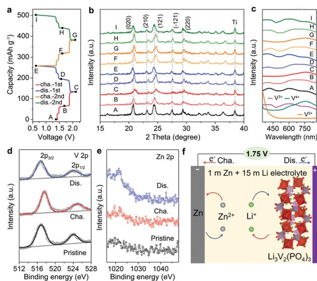
**Fig. 4** (a) Voltage profiles during the initial two cycles. (b) XRD patterns and (c) UV-vis spectra at selected states (points A-I marked in (a)). XPS spectra of (d) V 2p and (e) Zn 2p regions. (f) Schematic illustration of the Zn//1 m Zn + 15 m Li/LVP battery chemistry.
