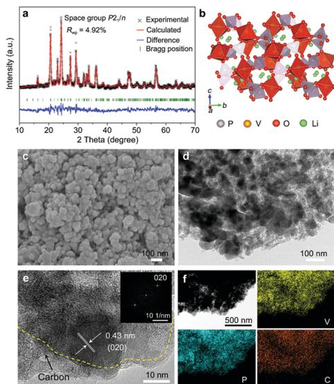
**Fig. 1** (a) Rietveld refined XRD pattern of the as-prepared LVP. (b) Schematic illustration of the LVP crystal structure. (c) SEM image. (d) TEM and (e) HRTEM images, with the inset presenting the corresponding FFT pattern. (f) STEM image with elemental mapping images.
