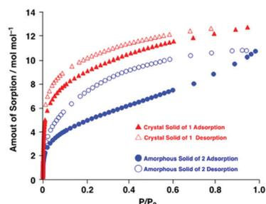
Fig. 6 Results of  $\text{CO}_2$  sorption by **1** at  $-78^\circ\text{C}$  in (a) the crystalline solid (red triangles) and (b) the ground amorphous state after 40 min (blue circles). Both samples were first dried *in vacuo* at  $100^\circ\text{C}$  for 12 h.
