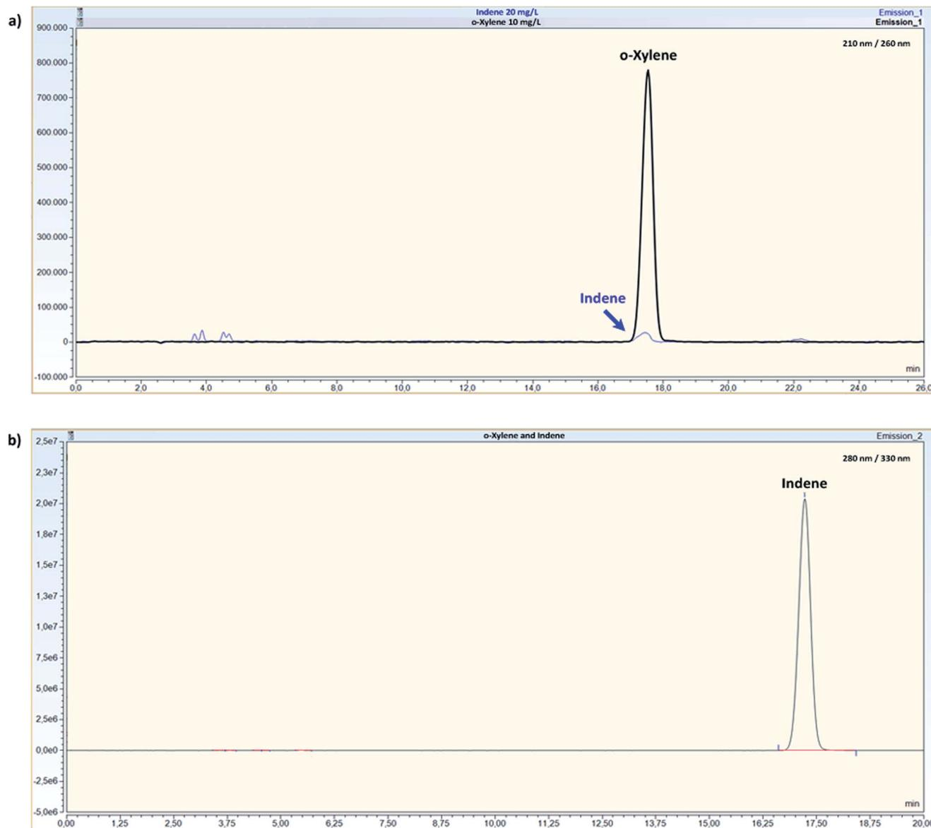
Fig. 3 Chromatogram of *o*-xylene ( $10 \text{ mg L}^{-1}$ ) detected at 210/260 nm. An interference with indene ( $20 \text{ mg L}^{-1}$ ) can be seen as a small peak (a) and chromatogram of only indene at 280/330 nm (b) by the use of a HPLC-FLD.
