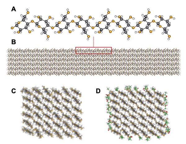
Fig. 1 Cellulose structure: the glucan chain (A) and a model cellulose nanofibril (B). Cross sections showing the crystalline  $I_{\beta}$  structure of unmodified (C) and surface acetylated (D) cellulose. Carbon atoms are shown in black, oxygen atoms in orange, and hydrogen atoms in white. Carbon and oxygen atoms of surface acetyl groups are shown in green and red, respectively.
