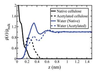
**Fig. 6** The interphase region in cellulose–water. Mass distribution profiles of water are presented perpendicular to the cellulose surface at DS 0 (native cellulose, solid lines) and DS 1 (acetylated cellulose, dashed lines). The *y*-axis shows the density of cellulose (black) and water (blue) relative to that of bulk water density (horizontal line at larger distances *z*). The *x*-axis is the distance *z* from the cellulose surface, measured (quite arbitrarily) from the first cellulose peak.
