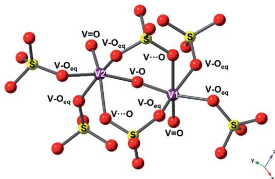
Fig. 7 Local environment of V(1) and V(2) atoms in  $V_2O_3(SO_4)_2$ , showing the different paths used in the EXAFS fitting model ( $(V=O) + (V-O) + (V-O_{eq}) + (V\cdots O) + (V-O-S)$ ), with the vanadium atoms shown as purple spheres, oxygen atoms as red spheres and sulfur atoms as yellow spheres.
