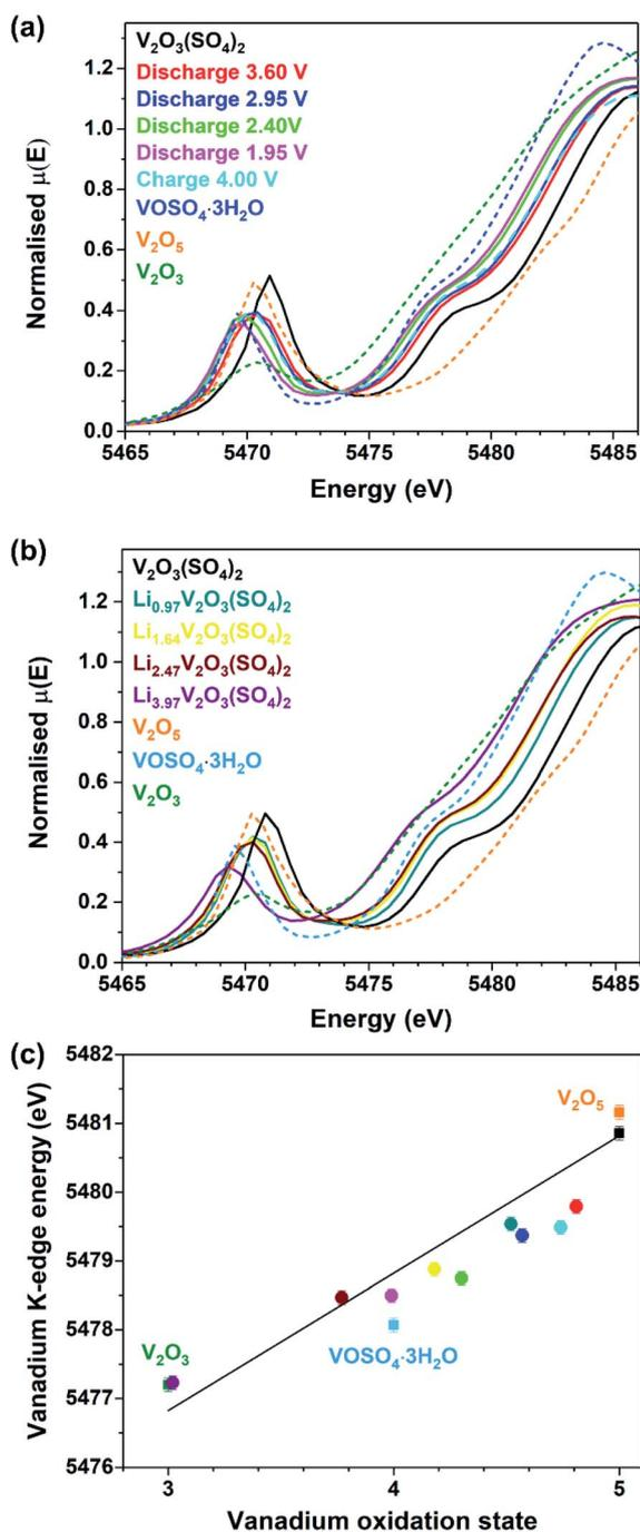
Fig. 5 Vanadium K-edge XANES data showing (a) normalised spectra for the  $V_2O_3(SO_4)_2$  electrodes at various states of discharge and charge compared to the reference materials,  $V_2O_5$ ,  $VOSO_4 \cdot 3H_2O$  and  $V_2O_3$ , (b) normalised spectra for the chemically lithiated  $V_2O_3(SO_4)_2$  samples compared to the reference materials and (c) vanadium K-edge energy (at half-height) as a function of oxidation state.
