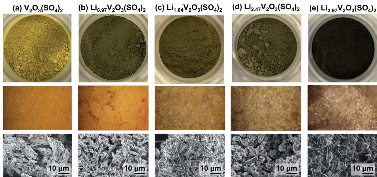
Fig. 4 Photographs (top), optical microscopy images (middle) and SEM micrographs (bottom) showing the colours and morphologies of (a) V<sub>2</sub>O<sub>3</sub>(SO<sub>4</sub>)<sub>2</sub>, (b) Li<sub>0.97</sub>V<sub>2</sub>O<sub>3</sub>(SO<sub>4</sub>)<sub>2</sub>, (c) Li<sub>1.64</sub>V<sub>2</sub>O<sub>3</sub>(SO<sub>4</sub>)<sub>2</sub>, (d) Li<sub>2.47</sub>V<sub>2</sub>O<sub>3</sub>(SO<sub>4</sub>)<sub>2</sub> and (e) Li<sub>3.97</sub>V<sub>2</sub>O<sub>3</sub>(SO<sub>4</sub>)<sub>2</sub>.
