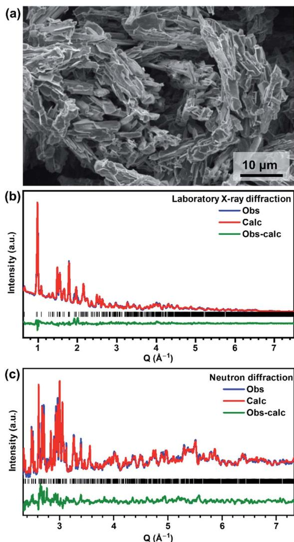
Fig. 1 (a) SEM micrograph of  $\text{V}_2\text{O}_3(\text{SO}_4)_2$ , (b) laboratory X-ray diffraction Rietveld fit and (c) neutron diffraction Rietveld fit for  $\text{V}_2\text{O}_3(\text{SO}_4)_2$  using the structural model published by Richter *et al.* as the starting model.<sup>23</sup>
