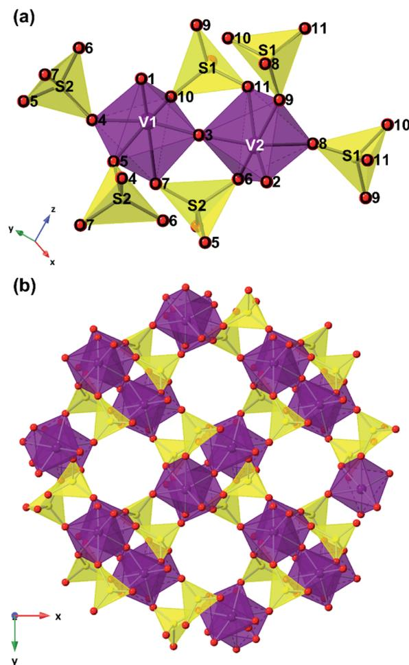
Fig. 2 Structural model of  $\text{V}_2\text{O}_3(\text{SO}_4)_2$  showing (a) the  $[\text{V}_2\text{O}_3]^{4+}$  subunit made up of pairs of vanadium octahedra (purple polyhedra) linked to each other by a bridging oxygen atom (red spheres) and two bridging  $\text{SO}_4$  tetrahedra (yellow polyhedra) and (b) the open channels down the  $c$ -axis.
