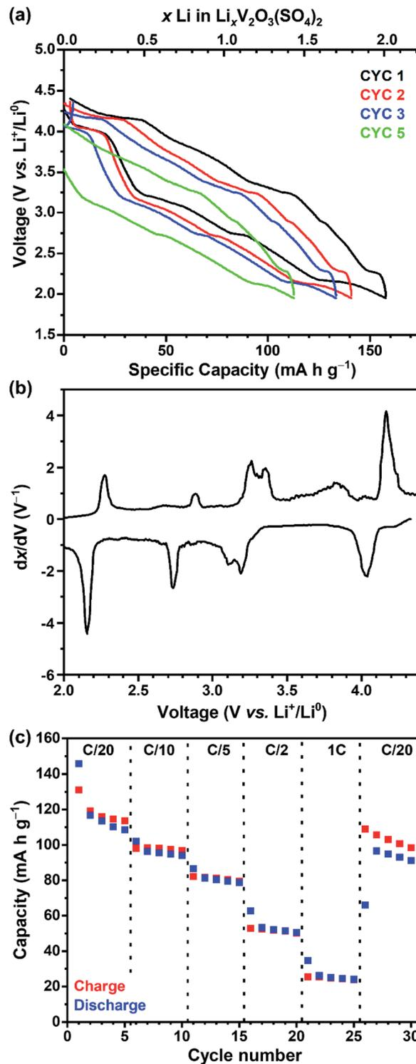
Fig. 3 (a)  $\text{V}_2\text{O}_3(\text{SO}_4)_2||\text{Li}$  cell cycled at a rate of C/20 between 4.20 V and 1.95 V showing the voltage–capacity curve for the first (black), second (red), third (blue) and fifth cycles (green), (b) the derivative  $\text{d}x/\text{d}V$  curve of the first cycle and (c) the specific capacity versus different C-rates (C/20, C/10, C/5, C/2, 1C) of  $\text{V}_2\text{O}_3(\text{SO}_4)_2$  cycled between 4.20 V and 1.95 V vs.  $\text{Li}^+/\text{Li}^0$ .
