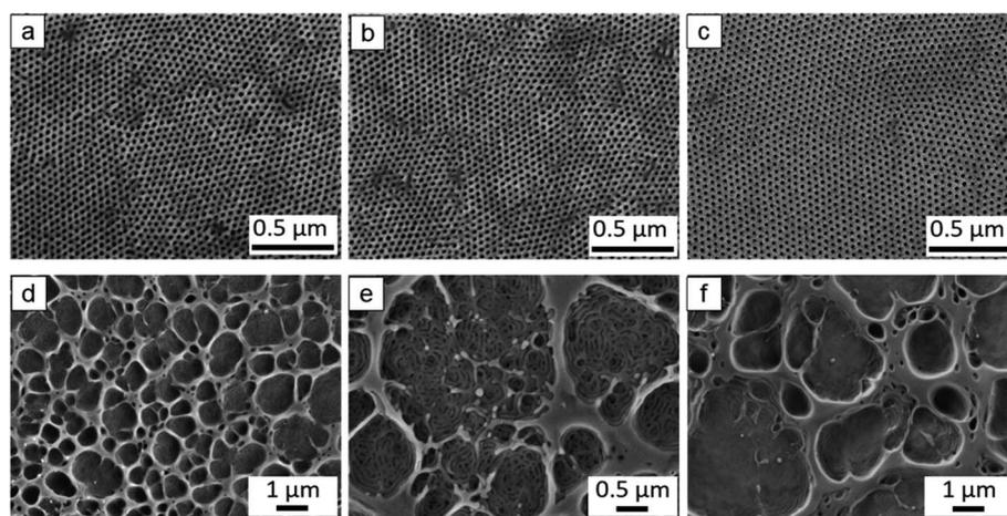
Fig. 3 Secondary electron (SE) images of SEM: top surface and bottom interface of P4 membranes cast from 25 wt% solution in THF/DMF/DOX 2 : 1 : 1 wt% (a and d) in the 32 °C H<sub>2</sub>O bath, (b and e) in the non-solvent bath of methanol/H<sub>2</sub>O (2 : 8 vol%), (c and f) with 6 wt% (as P4) PEG400 as the porogen. All of the evaporation time is  $t = 5$  s.
