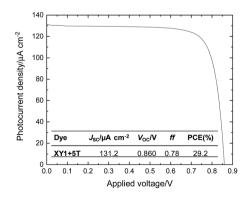
Fig. 8 J-V curve of the best XY1 + 5T DSSC at 1000 lux. The inset shows the measured values of the cell parameters
