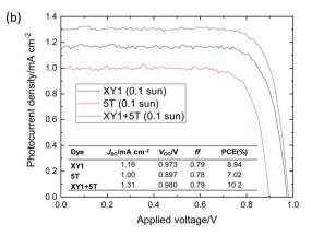
Fig. 4 J-V curves of the best DSSCs at (a) 1 sun and (b) 0.1 sun. The insert shows the measured values of the cell parameters.
