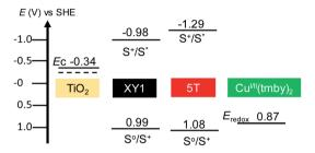
Fig. 2 Energy diagram of the dyes used in this study, in comparison with the  $TiO_2$  anode and  $Cu^{I/II}(tmby)_2$  electrolyte. All state levels are described in volts. The values were taken from the literature.<sup>38,41,48</sup>
