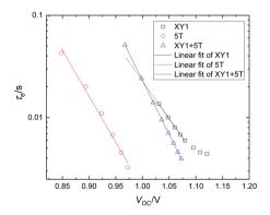
Fig. 6 Electron lifetime ( $\tau_e$ ) of the best DSSCs (XY1: black square; 5T: red circle; XY1 + 5T: blue triangle), plotted against  $V_{OC}$  at different light intensities. The solid lines are linear fits of the linear region. The dashed line for XY1 is an extension of the linear fit, which intercepts the linear fit of XY1 + 5T at  $V_{\rm OC} \sim$  1.0016 V.
