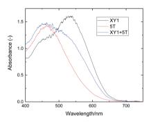
Fig. 3 UV-vis absorption spectra of XY1-, 5T- and XY1 + 5T-sensitized transparent  $TiO_2$  films. Baseline was a non-sensitized  $TiO_2$  film.
