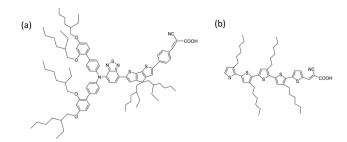
Fig. 1 Molecular representation of (a) XY1 dye and (b) 5T dye used in this study.
