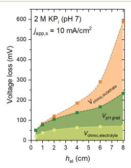
Fig. 2 Contribution of the electrolyte ohmic loss ( $V_{\rm ohmic,electrolyte}$ ), the pH gradient loss ( $V_{\rm pH\ grad}$ ), and the substrate ohmic loss ( $V_{\rm ohmic,substrate}$ ) as a function of the height of the electrode ( $h_{\rm el}$ ). The electrolyte is 2 M KP<sub>i</sub> buffer (pH 7).  $J_{\rm app,s}=10$  mA cm<sup>-2</sup>,  $v_{\rm in}=0.27$  cm s<sup>-1</sup>,  $\sigma_{\rm el}=10^5$  S m<sup>-1</sup>,  $h_{\rm cell}=10$  cm, and  $w_{\rm cell}=3$  cm.
