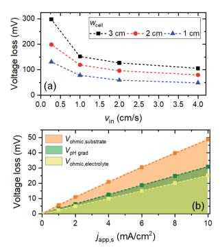
Fig. 6 (a) Total voltage losses for the 8 cm electrode with varying inlet velocities ( $v_{\rm in}$ ) and cell widths ( $w_{\rm cell}$ );  $j_{\rm app,s}=10$  mA cm $^{-2}$ ,  $d_{\rm contact}=1$  cm. (b) Contribution of voltage losses at varying current densities;  $w_{\rm cell}=1$  cm,  $v_{\rm in}=4$  cm s $^{-1}$ ,  $d_{\rm contact}=1$  cm. In all cases, the electrolyte is 2 M KP $_{\rm i}$  buffer (pH 7),  $h_{\rm el}=8$  cm, and  $h_{\rm cell}=10$  cm.
