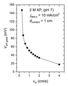
Fig. 5 Voltage loss associated with pH gradient ( $V_{\rm pH\ grad}$ ) as a function of the inlet velocity  $(v_{in})$ . The electrolyte is 2 M KP<sub>i</sub> buffer (pH 7).  $j_{app,s} =$ 10 mA cm<sup>-2</sup>,  $d_{\text{contact}} = 1$  cm,  $h_{\text{el}} = 8$  cm,  $h_{\text{cell}} = 10$  cm, and  $w_{\text{cell}} =$
