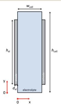
Fig. 1 Schematic of the computational domain consisting of the liquid electrolyte and the two solid electrodes:  $h_{cell} = cell$  height,  $w_{cell} = cell$ width,  $h_{\rm el}=$  electrode height,  $d_{\rm el}=$  electrode thickness.
