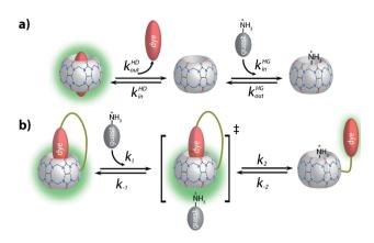
Fig. 9 (a) Schematic representation of a  $S_N1$ -type-mechanism for the guest-exchange process on analyte-induced conformational changes of non-covalent CB7 $\supset$ dye reporter pair complexes; (b) schematic representation of a  $S_N2$ -type-mechanism for the guest-exchange process on analyte-induced conformational changes of CB7–dye conjugates.
