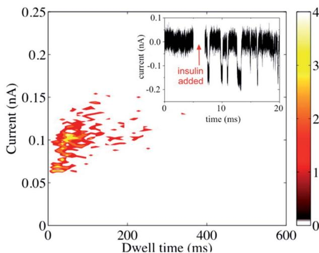
Fig. 5 Resistive-pulse sensing of insulin molecules with a metallized nanopore. Scatter plot and the current–time recording (inset) before and after the addition of the  $0.1 \text{ mg mL}^{-1}$  insulin to the solution containing 0.1 M KCl and 40 mM HCl.  $V = -400$  mV. Reprinted with permission from ref. 53; copyright 2015, American Chemical Society.
