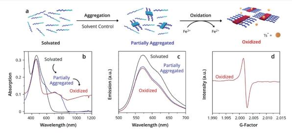
Fig. 1 Oxidation-promoted self-assembly. (a) Schematic depicting the aggregation and oxidation of  $PTh_{80}$ -b- $PTe_{60}$  by  $FeTs_3$  to oxidized micelles. Demonstrated by (b) UV-Vis-NIR spectra, (c) PL spectra, and (d) EPR spectra. All solutions prepared at 0.05 mg mL<sup>-1</sup>  $PTh_{80}$ -b- $PTe_{60}$ .
