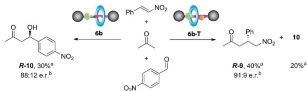
Scheme 3 Michael versus aldol addition of acetone using rotaxane 6b as the catalyst in the presence or absence of N -hexylthymine ( T ). Reaction conditions: p -nitrobenzaldehyde (1 equiv.), trans - \beta -nitrostyrene (1 equiv.), acetone (1.5 equiv.), catalyst 6b (10 mol%), N -hexylthymine (5 equiv., if required), \text{CH}_2\text{Cl}_2 (0.25 M), 25 °C, 5 days. a Determined by ^1\text{H} NMR from the crude reaction. b e. r. determined by HPLC using a Daicel ChiralPak AS-H column.
