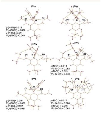
Fig. 3 Atom in molecules (AIM) analysis results based on X-ray geometries of  $2^{\text{Me}}a$ -b,  $2^{\text{iP}}ra$ -b,  $3^{\text{Me}}a$  and  $3^{\text{iP}}ra$  showing bond paths between the central nitrogen and the carbonyl oxygen, calculated at the RCAM- and UCAM-B3LYP-D3/def2-SVP levels in 2 and 3, respectively.
