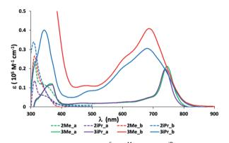
Fig. 1 Absorption spectra of  $10^{-5}$  M  $2^{Me}a$ -b and  $2^{iPr}a$ -b (dashed line) and  $3^{Me}a$ -b and  $3^{iPr}a$ -b (solid line) in  $CH_2Cl_2$  at  $25\,^{\circ}C$ .
