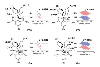
Fig. 5 Observed (bottom) and simulated (top) EPR spectra of  $3^{Me}a-b$  and  $3^{iPr}a-b$  in  $CH_2CI_2$  solution at 25 °C. Spin Hamiltonian parameters estimated from simulation are labelled in MHz (Table S3†).
