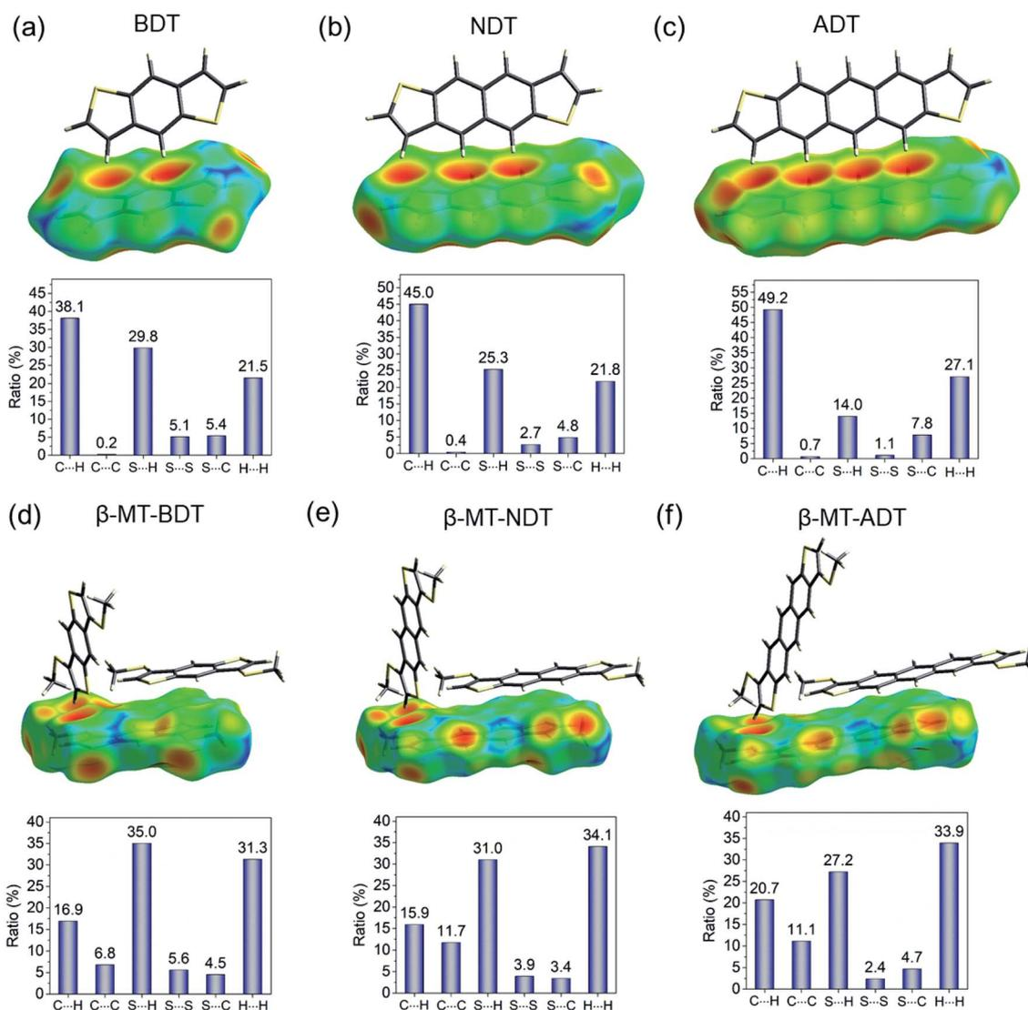
Fig. 4 Hirshfeld surface analysis of (a) BDT, (b) NDT (CCDC: 1899660), (c) ADT, (d)  $\beta$ -MT-BDT, (e)  $\beta$ -MT-NDT, and (f)  $\beta$ -MT-ADT, which illustrates the distance ( $d_e$ ) from the surface to the nucleus of external atoms in the adjacent molecules in a red-green-blue colour scheme.
