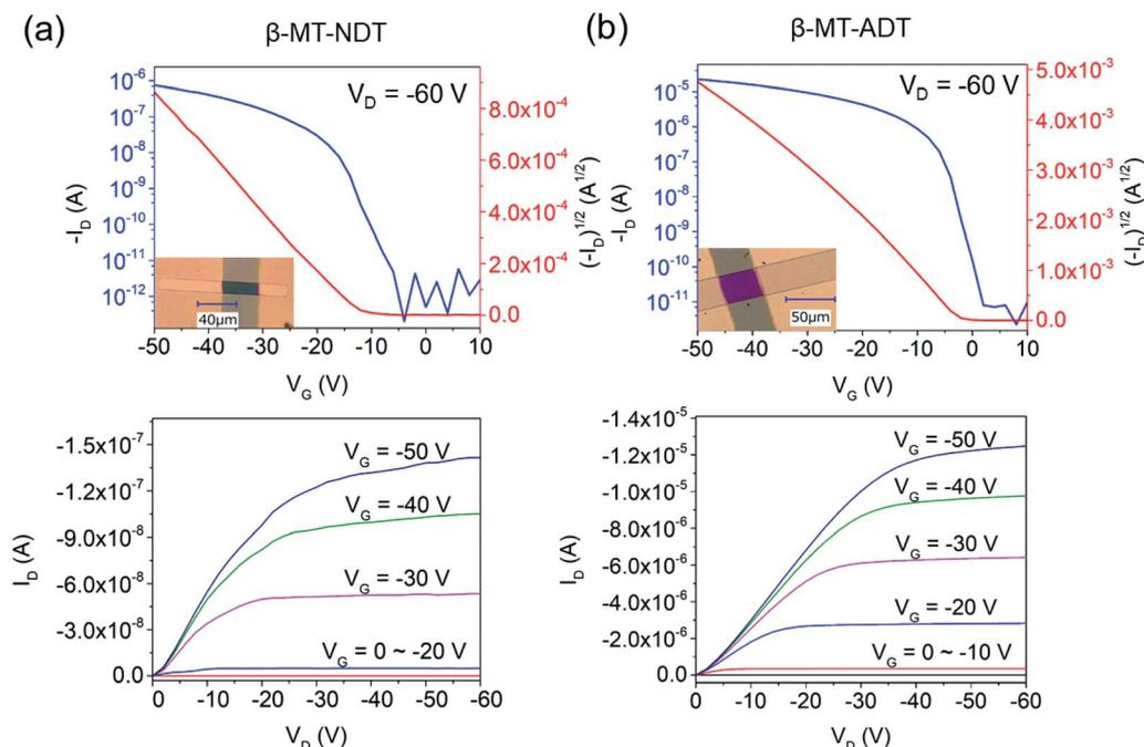
Fig. 3 Transfer (top) and output (bottom) curves of SC-OFETs (a)  $\beta$ -MT-NDT and (b)  $\beta$ -MT-ADT.
