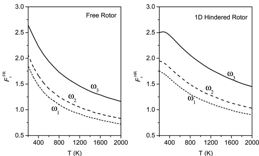
Fig. 9 Torsional anharmonicity factors for FR and HR treatments by different assignments of the normal modes to the torsion;  $\omega_1$ ,  $\omega_2$  and  $\omega_3$  denote the normal modes of frequencies  $66.6$ ,  $78.7$ , and  $109.1\text{ cm}^{-1}$ , respectively. Each curve is labeled by the vibrational mode for which the QH approximation is replaced by the torsional partition function.
