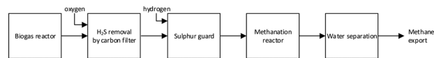
Fig. 1 Block diagram of the steps required when upgrading raw biogas to methane.
