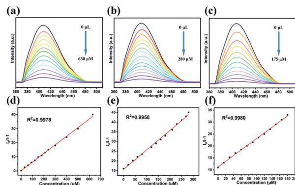
Fig. 5 Fluorescence spectra of LCP 1 dispersed in different concentrations of Fe<sup>2+</sup> (a), Hg<sup>2+</sup> (b) and Fe<sup>3+</sup> (c). The S–V plot of LCP 1 at different concentrations of Fe<sup>2+</sup> (d), Hg<sup>2+</sup> (e) and Fe<sup>3+</sup> (f).
