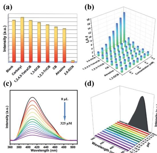
Fig. 4 (a) Fluorescence intensity of LCP 1 dispersed in OCPs. (b) The fluorescence intensity of  $I_0/I$  of LCP 1 vs. the concentration of various pesticides. (c) Luminescence titration of LCP 1 at different concentrations of 2,6-DCN in THF solution. (d) The luminescence intensity in the pH range of 2.0–12.0 of 2,6-DCN.
