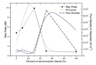
Fig. 11 Relations among the titania semiconductor content of the composites, peak reflection loss of the composites, and flux density in the absorbers.
