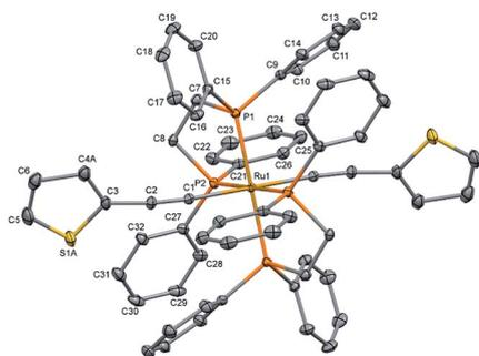
Fig. 2 Molecular structure of *trans*-[Ru(dppe)<sub>2</sub>(T)<sub>2</sub>] (all hydrogen atoms are omitted for clarity). The thermal ellipsoids are drawn at the 20% probability level.
