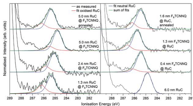
Fig. 7 Ru 3d core level XPS spectra of RuC–F<sub>6</sub>TCNNQ interfaces; left: F<sub>6</sub>TCNNQ as bottom layer with stepwise deposition of RuC; right: opposite sequence. The fit obtained from the neutral spectrum (bottom right) is shown in blue. All other spectra can be reconstructed by a superposition of the neutral spectrum and a second contribution which is assigned to oxidised molecules (red). Spectra were fitted with PseudoVoigt profiles with the software Fityk.<sup>25</sup>
