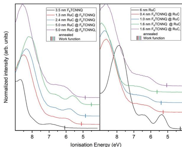
**Fig. 9** UP spectra of valence region of RuC–F<sub>6</sub>TCNNQ interfaces; left: F<sub>6</sub>TCNNQ as bottom layer with stepwise deposition of RuC; right: opposite sequence. The measured work functions for each deposition step are indicated by vertical lines.
