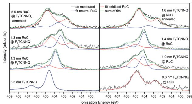
**Fig. 8** N 1s XPS spectra of RuC–F<sub>6</sub>TCNNQ interfaces; left: F<sub>6</sub>TCNNQ as bottom layer with stepwise deposition of RuC; right: opposite sequence. The neutral spectrum (bottom right) and the reduced spectrum (bottom left) were fitted by PseudoVoigt profiles (blue and red) curves. All other spectra could be reconstructed by a superposition of those two contributions.
