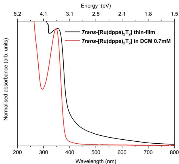
Fig. 3 Absorption spectra of a spin coated RuC film on a glass substrate (black) and a DCM solution of 0.7 mmol L<sup>-1</sup> RuC.
