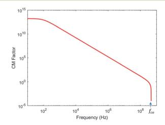
Fig. 3 Clausius—Mossotti factor as a function of frequency for Ni NWs in an ethanol suspension.
