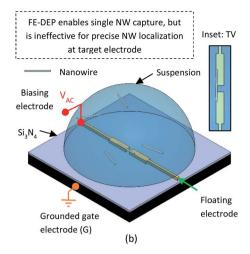
Fig. 1 Schematic diagram of an on-chip platform based on: (a) magnetic field assisted floating electrode DEP design, (b) floating electrode DEP design. The inset in (a) and (b) show the Top View (TV) of respective NW deposition from magnetic field assisted FE-DEP and FE-DEP process.
