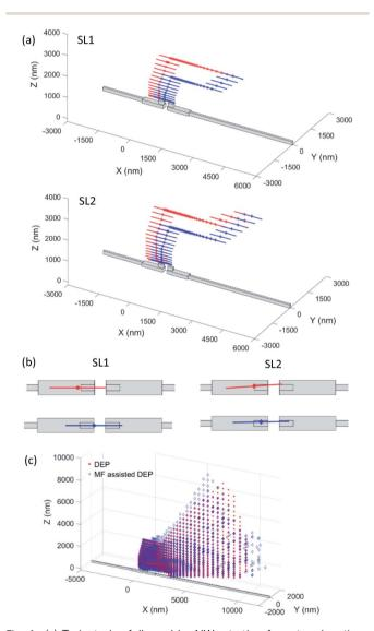
Fig. 4 (a) Trajectories followed by NWs starting from two locations [SL1 (3153, 0, 2277) and SL2 (4114, 25, 3588)] in the simulation workspace during pure FE-DEP (red NWs) and magnetic-field assisted FE-DEP (blue NWs); (b) corresponding final deposition location and orientation for NWs starting from SL1 and SL2; and (c) starting workspace locations that yield high precision NW deposition on Co nanomagnets in a bridging configuration within 30 seconds.
