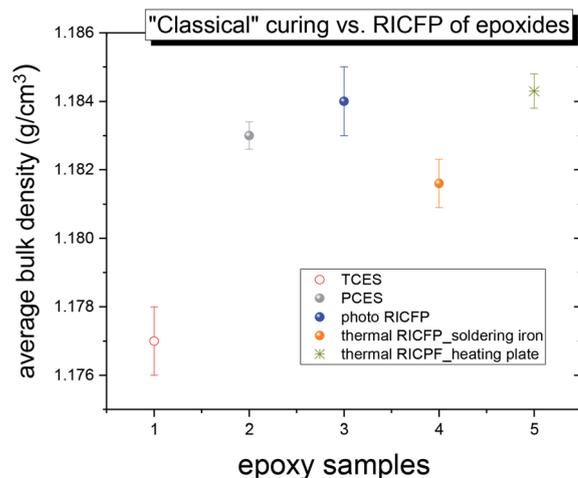
Fig. 2 The average bulk density of the discs determined for the “classically” thermally- and photo-cured epoxy samples, *i.e.* TCES (○), PCES (●), as well as RICFP of BADGE/PAG + TPED induced by UV light (photo RICFP) (●) or heat (thermal RICFP, induced by the soldering iron (●) or the heating plate (\*)).
