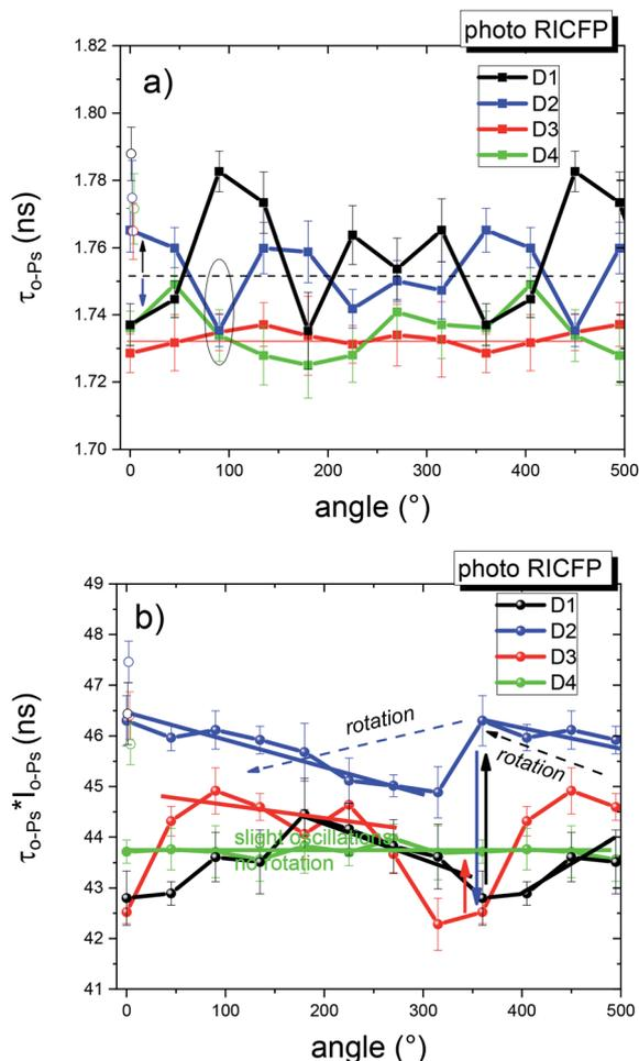
Fig. 14 2D angular dependence of (a) *o*-Ps lifetime and (b)  $\tau_{o-Ps} \times I_{o-Ps}$  for the discs D1–D4 of photo RICFP induced by UV light, determined at a distance of 3 mm from the edge of the discs, with the inclusion of the values in the core of the discs (open symbols).
