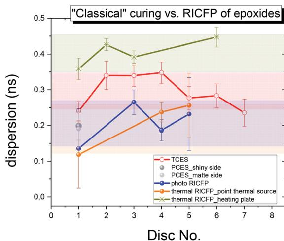
**Fig. 10** The average dispersion of the *o*-Ps lifetime in the core of the all discs along the studied samples prepared by the “classical” thermal and photo curing procedures and the frontal polymerization induced by UV light and two types of heaters.
