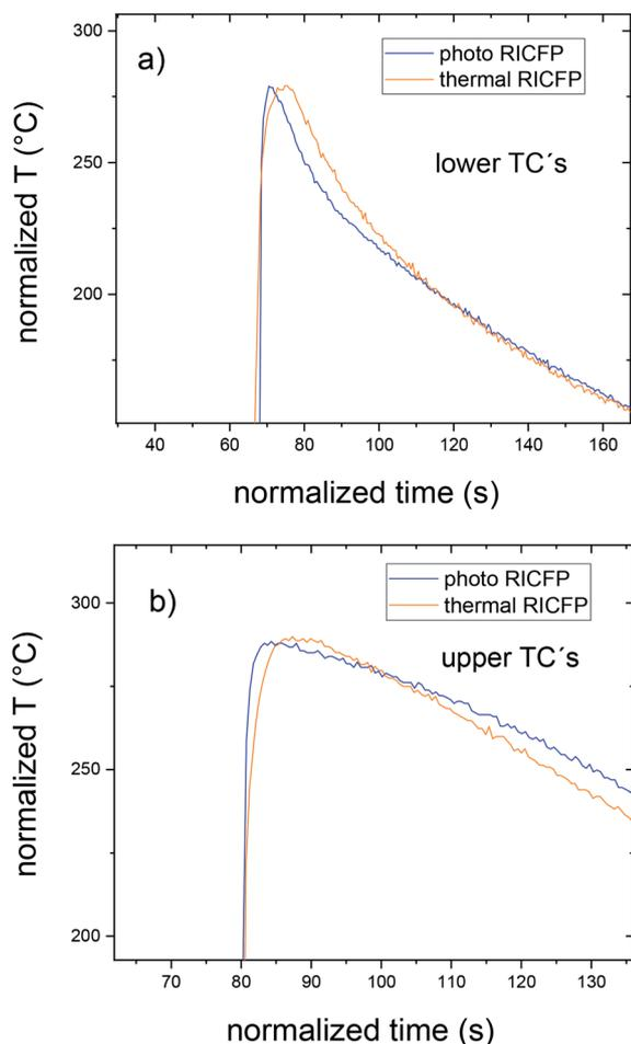
**Fig. 5** Mutual comparison of the temperature profiles of photo- and thermally-induced RICFP in the middle of the cylinder for (a) the lower and (b) upper thermocouples. The temperature profile of thermal RICFP is normalised to the time and amplitude of photo RICFP.
