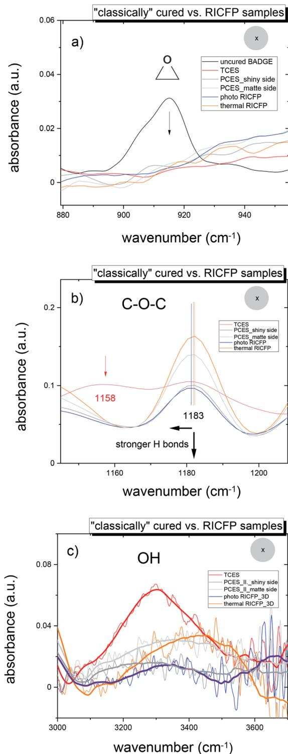
Fig. 1 ATR/FTIR results of the 5<sup>th</sup> disc of “classically” thermally- and photo-cured samples from series I (TCES, PCES) and the 3<sup>rd</sup> disc of photo and thermal RICFP samples, for the range (a) 880–940  $\text{cm}^{-1}$ , with inclusion unured reference (BADGE/PAG + TPED) (b) 1160–1200  $\text{cm}^{-1}$  and (c) 3000–3600  $\text{cm}^{-1}$ .
