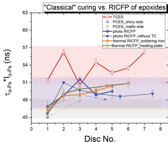
Fig. 11 Free volume fraction parameter ( $\tau_{o-Ps} \times I_{o-Ps}$ ) for a series of studied epoxy samples cured "classically" and by RICFP. In a series of RICFP-based samples, only photo induced RICFP by UV light exhibited, after a slight increase of void fraction, a decrease in void fraction.
