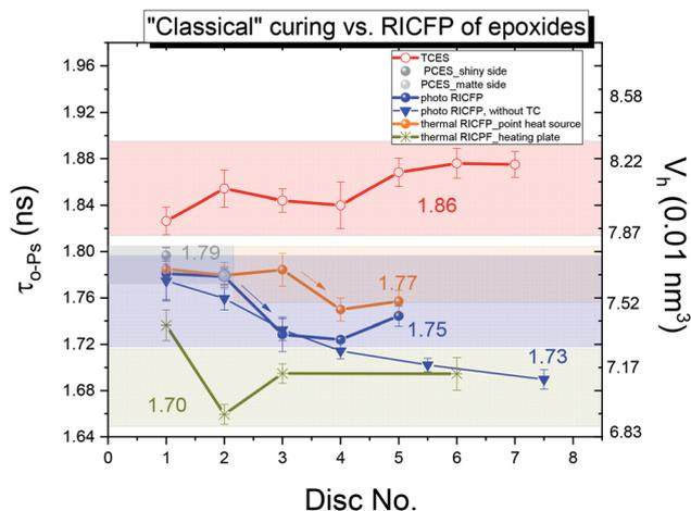
**Fig. 9** The average *o*-Ps lifetime dependence and corresponding size of free volume ( $V_h$ ) in the core of all discs, along the axes of the investigated samples. Two comparable data sets of photo RICFP-based samples, prepared both in the presence of TCs and in the absence of TCs, confirmed that TCs had no influence on the microstructure in the middle of the front.
