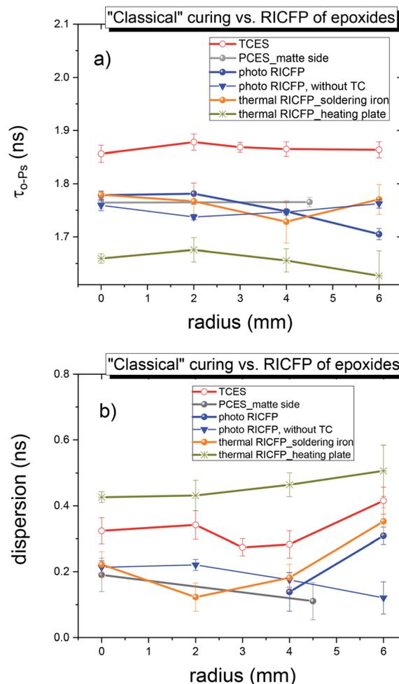
Fig. 12 Radial dependence of (a) average *o*-Ps lifetime and (b) its dispersion for "classically" photo-cured sample (PCES) and 2<sup>nd</sup> disc of cylindrical samples, *i.e.* "classically" cured TCES sample and RICFP samples induced by UV light, soldering iron and heating plate.
