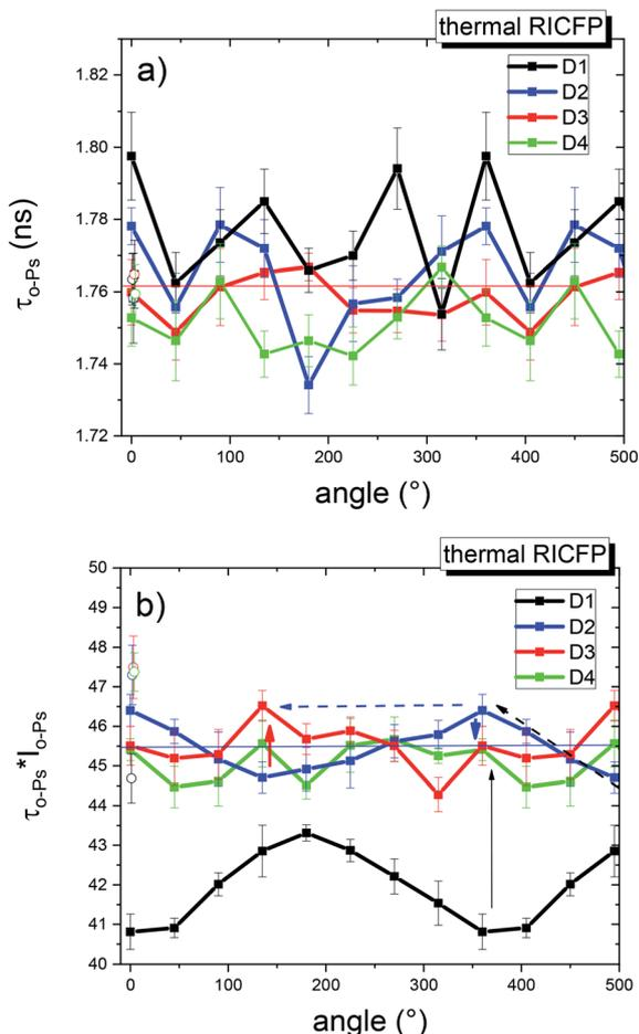
Fig. 15 2D angular dependence of (a) the average *o*-Ps lifetime and (b)  $\tau_{o\text{-Ps}} \times I_{o\text{-Ps}}$  for discs D1–D4 of thermal RICFP induced by soldering iron, determined at a distance of 3 mm from the edge of the discs, including the values in the core of the discs (open symbols).
