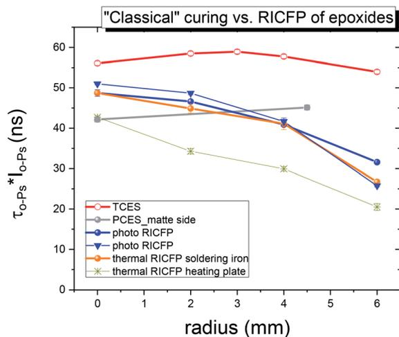
Fig. 13 Radial dependence of the free volume fraction parameter for “classically” photo-cured sample and the 2<sup>nd</sup> discs of the cylindrical samples, *i.e.* “classically” cured TCES sample and samples cured *via* RICFP induced by UV light, soldering iron and heating plate.
