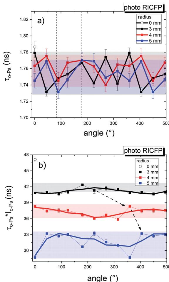
Fig. 17 2D angular dependence of (a) the average *o*-Ps lifetime and (b)  $\tau_{o\text{-Ps}} \times I_{o\text{-Ps}}$  for four different radii of the “crater”-shaped end of the photo-induced RICFP sample.
