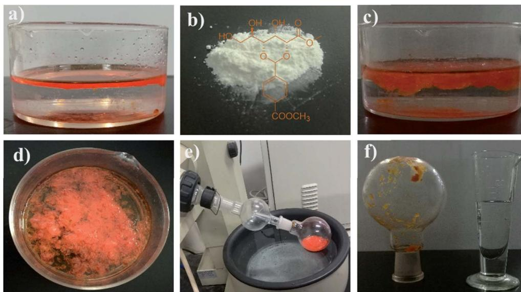
Fig. 3 Demonstration of aromatic solvents recovery. (a) Biphasic system was prepared by adding 20 mL of toluene (dyed with Methyl Red) into 200 mL of water. (b) Powders of GAA-2. (c) 500 mg of gelator powders were dispersed over the solvent surface after being gently stirred at room temperature for 65 min. (d) Formation of a stable gel. (e) Distillation of toluene extracted from the gel. (f) Toluene was recycled from water by GAA-2.
