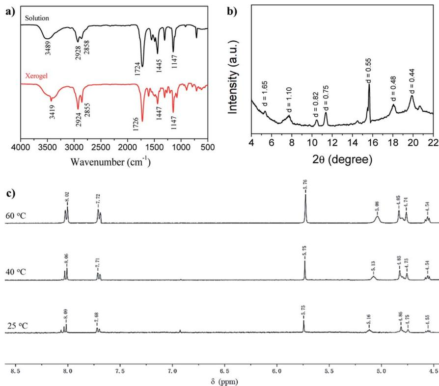
Fig. 1 (a) FTIR spectra of solution (0.1 mM) and xerogel (1.0% w/v) of **GAA-2** in acetonitrile. (b) WXR D spectra of **GAA-2** xerogels made from acetonitrile. (c) Change in  $^1\text{H}$  NMR chemical shift of hydroxyl and aromatic protons of gelator **GAA-2** in  $\text{CD}_3\text{CN}$  at different temperatures.
