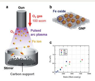
Fig. 1 (a) Process for producing SIOPs using the APD method. (b) Model of the deposited SIOPs on carbon materials. (c) Plots of the Fe loadings *versus* the shot count ratios (shot count/weight of supports:  $q^{-1}$ ).
