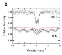
Fig. 5  $^{57}$ Fe Mössbauer spectra measured of (a) GNP $_{3666}$  and (b) GNP $_{10900}$  at 300 and 10 K. The gray curve denotes the fitting curve, where the red and blue curves stand for the paramagnetic and magnetic components, respectively.
