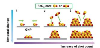
Fig. 7 Model for the growth of iron oxide nanoparticles on GNP. (1) Formation of iron oxide cores, (2) stacking of the  $FeO^+$  species on the  $Fe_2O_3$  cores and (3) growing of the particles with higher density to create large size of the nanoparticles.
