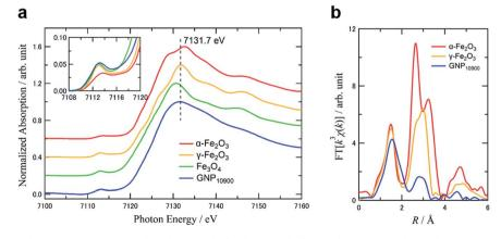
Fig. 4 (a) Normalized XANES spectra of GNP<sub>10900</sub> (blue),  $\alpha$ -Fe<sub>2</sub>O<sub>3</sub> (red),  $\gamma$ -Fe<sub>2</sub>O<sub>3</sub> (yellow), and Fe<sub>3</sub>O<sub>4</sub> (green). Inset shows the pre-edge peaks of all the samples. (b) Fourier transform of EXAFS spectra ( $k^3$ :  $\Delta k = 3-16$  Å<sup>-1</sup>).
