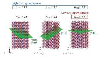
Fig. 5 Schematic of the lattice planes (green plane), values of surface energy ( $\alpha_{hkl}$ , nm $^{-2}$ ), and number of FeO $_6$ -broken bond per area ( $N_{hkl}$ , nm $^{-2}$ ) for the rod-shaped  $\epsilon$ -Fe $_2$ O $_3$  nanocrystals (Table S3 $\dagger$ ). Red, blue, and gray spheres in the crystal structure indicate the Fe at octahedral site, Fe at tetrahedral site, and O, respectively. Large  $\alpha$  and small N values indicate the easy-growth plane.
