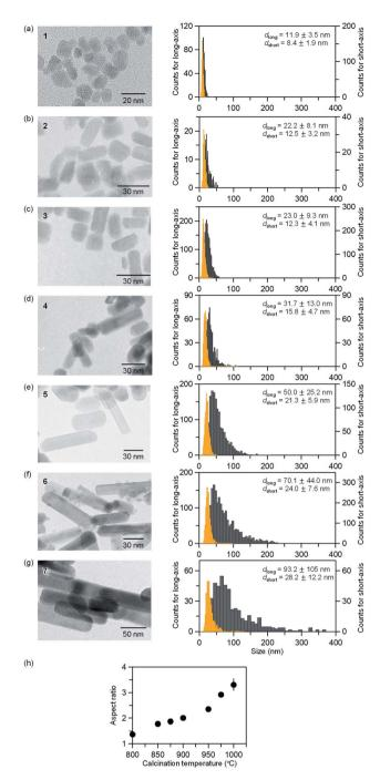
Fig. 3 TEM images for samples (a) 1, (b) 2, (c) 3, (d) 4, (e) 5, (f) 6, and (g) 7 (left). Particle size distributions of the long-axis ( $d_{\rm long}$ ) (gray) and the short-axis ( $d_{\rm short}$ ) (orange) for 1–7 (right). (h) Calcination temperature dependence of the aspect ratio estimated from the average size obtained by the TEM images.
