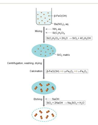
Fig. 1 Schematic of the synthesis for rod-shaped  $\epsilon\text{-Fe}_2\text{O}_3$  nanocrystals.
