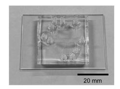
Fig. 2 Microfluidic device used in this experiment.
